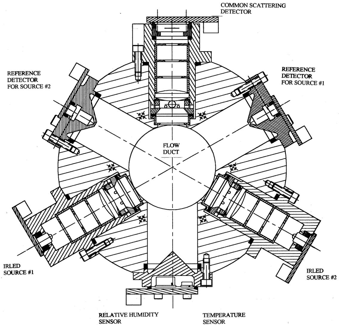
After these two beams traverse the sensing region within the flow duct, they enter their respective light traps at the end of which there are corresponding reference detectors that sense the intensity of each of the illumination beams. Feedback circuits ensure that the light output of both sources remains constant.
